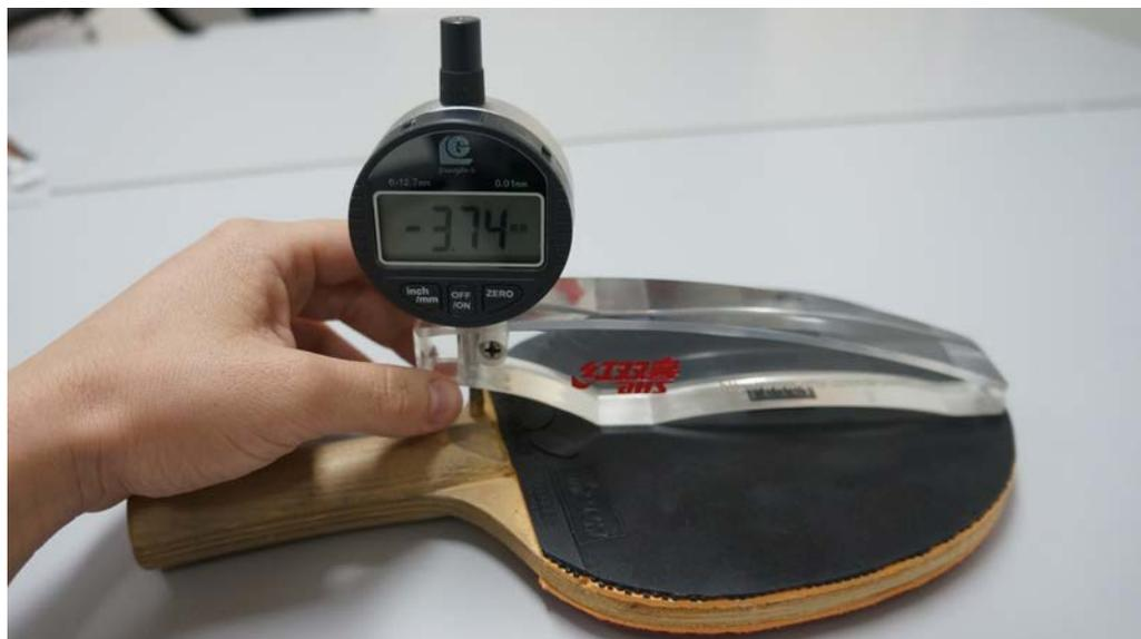
The diameter of the pin touching the blade shall be between 4.5 and 5.0 mm.
