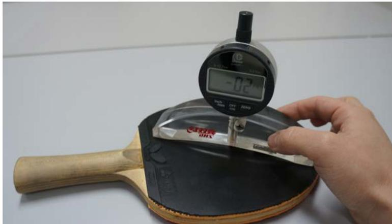
\*To determine the reason of the bad flatness of a racket, 2 quick checks are available:
